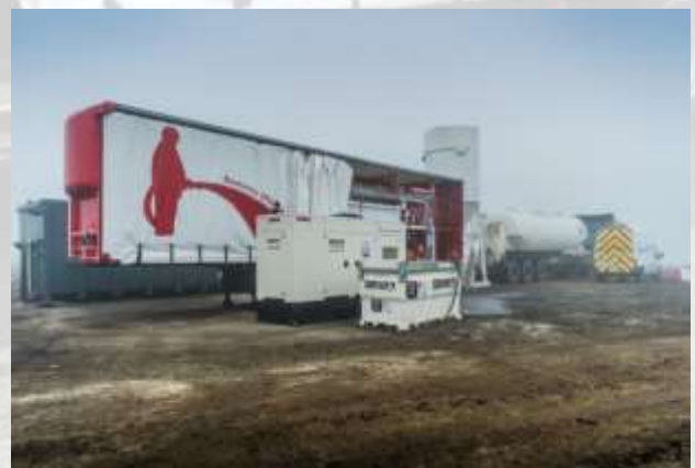
Site set up of 16m 3 batching mixing unit producing up to 300+m 3 /day
