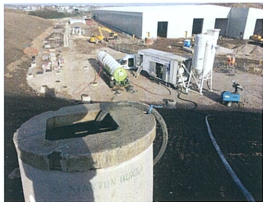
Foam Concrete batching plant with silo fully computerized densities from 400-1500 kgs strength 0.5-10 MPa @ 28 days.
